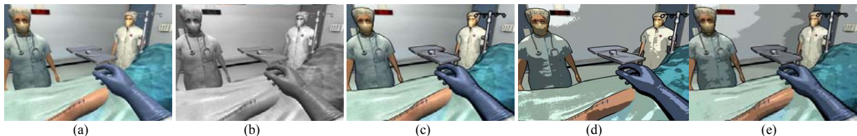
Fig. 1. Visual stimuli considered in this experiment. (a) Original (non-filtered), (b) gray-scale (removal of all color information), (c) outline (normal color but highlighting of edges), (d) cel-shading with three levels, and (e) cel-shading with six levels (i.e., color is divided into six discrete levels).
