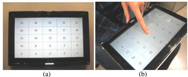
Figure 4. Portable touch-screen interface for automated registration of participant choices (a) and its operation (b).
