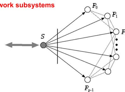
**Figure 1.** A central server,  $S$ , broadcasts audio stream data via high-bandwidth WiFi. A small network between phones nodes,  $P_p$ , supports the exchange of control data via low-bandwidth, low-power Bluetooth.
