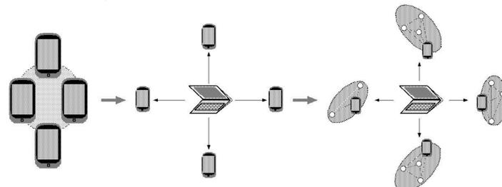
**Figure 2.** Phase 1: Master nodes are designated. Phase 2: Master nodes are assigned audio channels based on positions relative to the server. Phase 3: Additional phones can be recruited into piconets to support channel playback.
