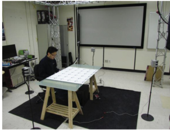
Fig. 4. “Diamond” loudspeaker setup. (a) The 36 virtual sound source positions and loudspeaker setup. (b) Actual setup.
