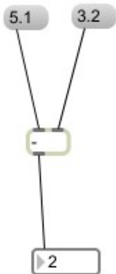
Figure 5.4: Float numbers get changed into integers if we use the basic operators.
