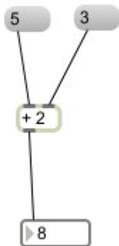
Figure 5.3 Over-riding an object's number by using the right inlet.
